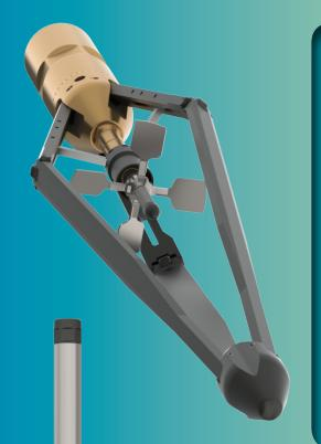
The Fullbore Flowmeter combine with our Temperature tool will allow you to run a production profile. The FBFM has a three arm spring loaded cage to center the impellers in multiple casing sizes so you only have to buy one tool. The blades design allow the impeller to work on small production rate wells do to the use of low friction bearings and the large cross sectional area. The tool is supplied with ancillary items that allow you to run in all casing sizes from 4-1/2" to 9-5/8".
